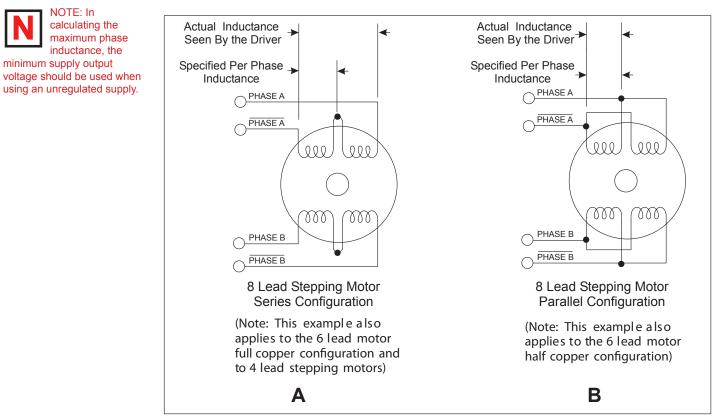
Figure 2.3.1 A & B: Per Phase Winding Inductance
